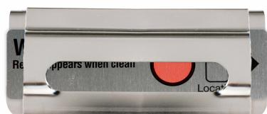
2. Position the Cleaning Monitor Holder face up inside a basket. Place basket on a shelf in the washer. Vary positions and shelves of Washer-Disinfector Cleaning Monitor placement cycle to cycle.
